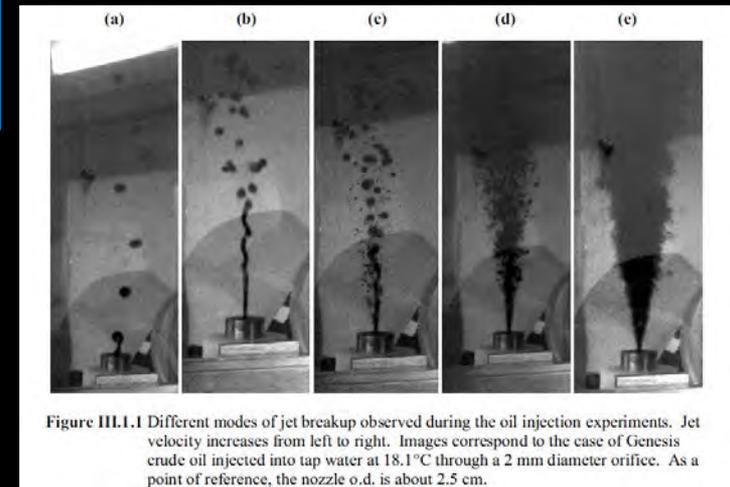
Figure III.1.1 Different modes of jet breakup observed during the oil injection experiments. Jet velocity increases from left to right. Images correspond to the case of Genesis crude oil injected into tap water at 18.1°C through a 2 mm diameter orifice. As a point of reference, the nozzle o.d. is about 2.5 cm.
