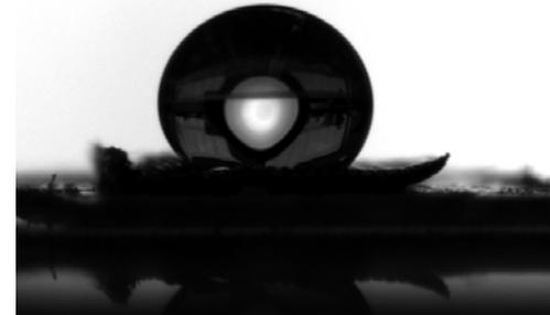
Static contact angle measurement using a water drop.
