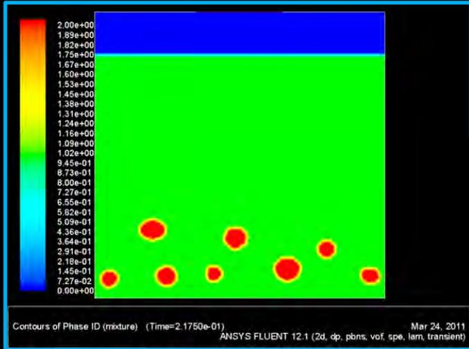
High fidelity (DNS-VOF) model captures dissolution while rising in water and evaporation on the surface followed by sinking to the ocean floor.
